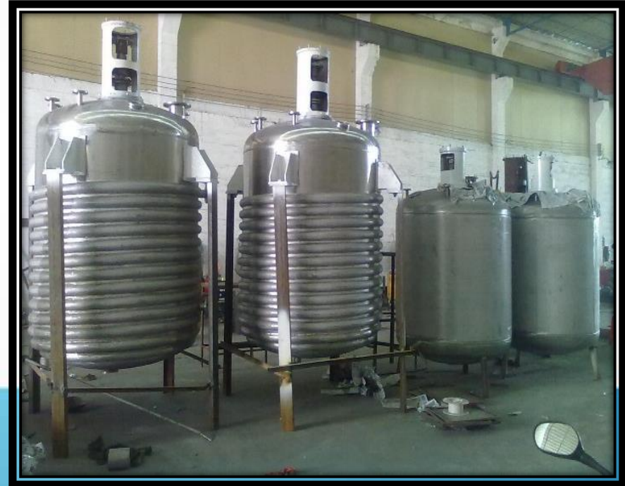
Jacketed Pipe Mixer
