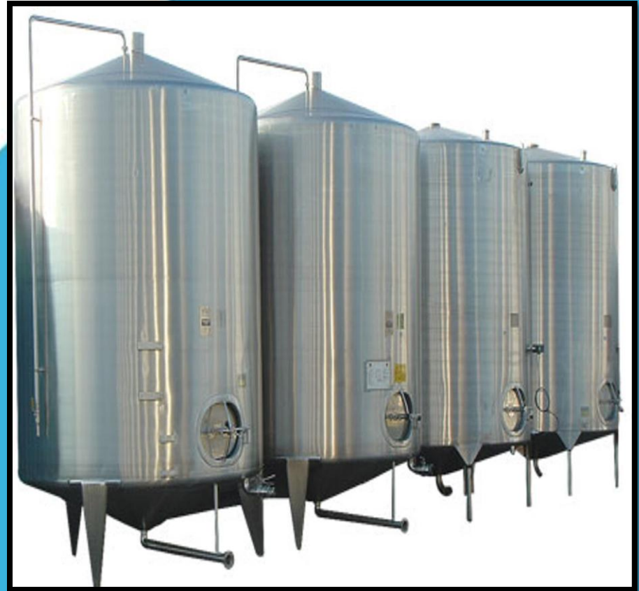
SETTLING TANK (MS)
