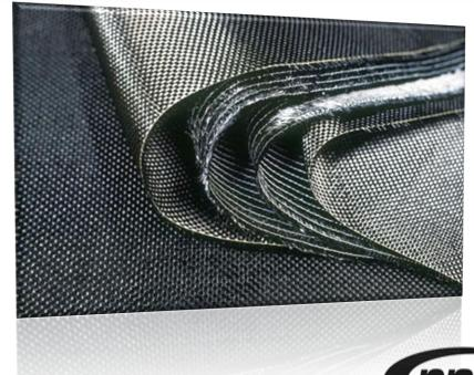
Carbon fiber material has a wide range of applications, as it can be formed at various densities in limitless shapes and sizes. Carbon fiber is often shaped into tubing, fabric, and cloth, and can be custom-formed into any number of composite parts and pieces.
